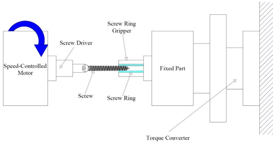
Fig. 4. Torsion test setup.
