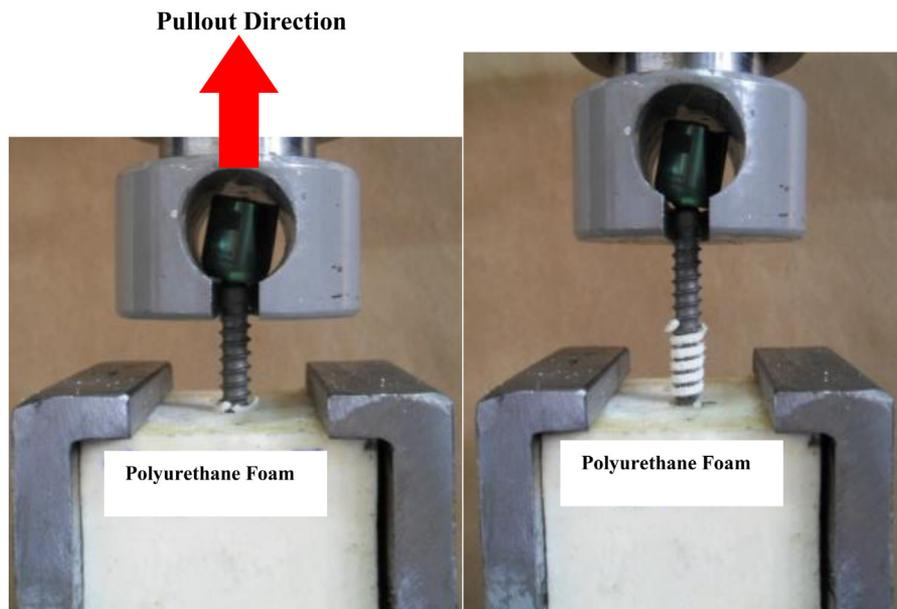
Fig. 3. Pullout test setup: before test (left) and after test (right).
