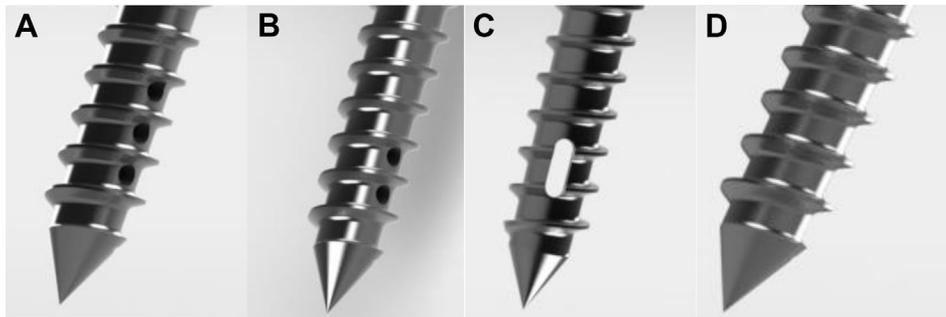
Fig. 2. Screws tips and radial hole/gap position. (A) Screw with 3 holes; (B) screw with 2 holes; (C) screw with gap; (D) non-cannulated screw.
