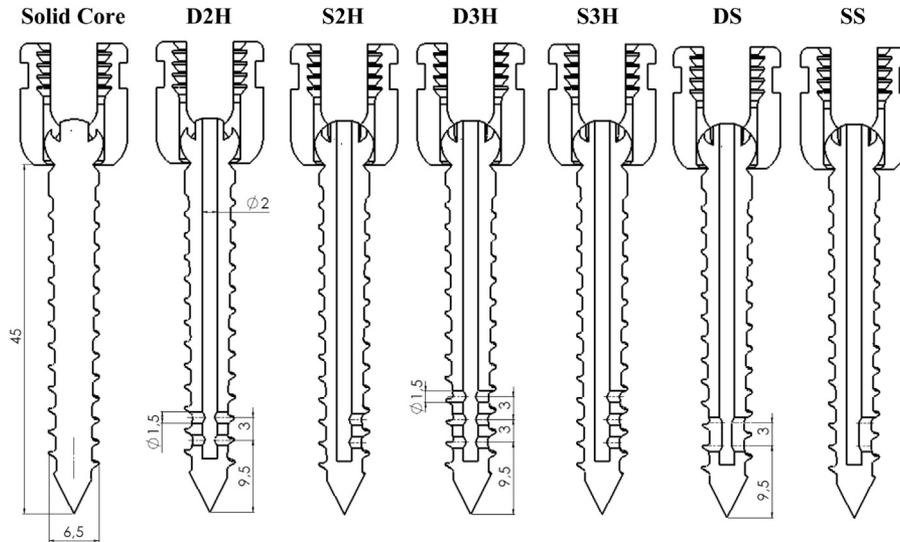
Fig. 1. Design parameters of screws (screw cross-sections). Solid Core, non-cannulated; D2H, 2 holes row bilaterally; S2H, 2 holes row unilaterally; D3H, 3 holes row bilaterally; S3H, 3 holes row unilaterally; DS, screw with gap bilaterally; SS, screw with gap unilaterally.
